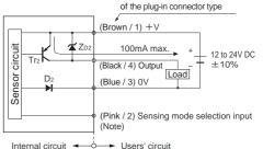
Symbols...D<sub>1</sub>, D<sub>2</sub> : Reverse supply polarity protection diode Z<sub>D1</sub>, Z<sub>D2</sub>: Surge absorption zener diode Tr1: NPN output transistor Tr2: PNP output transistor
