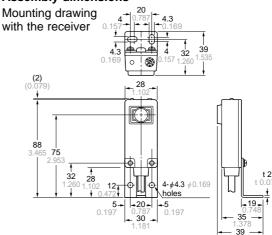
Material: Cold rolled carbon steel (SPCC) Two M4 (length 15 mm 0.591 in) screws with washers are attached.
