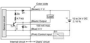
Note: The transmitter has only two power supply wires ( + V and 0 V).
