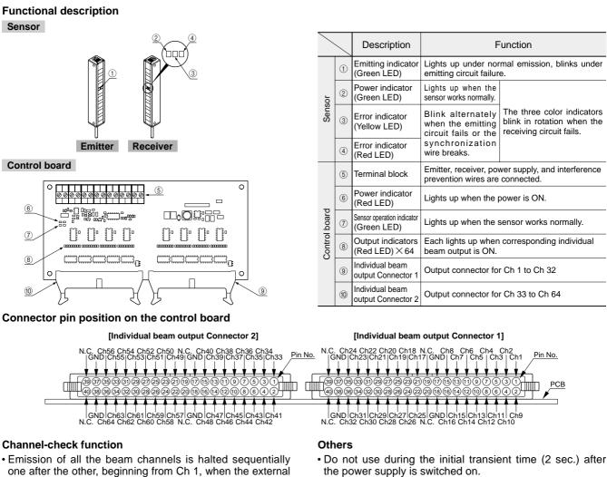
input (pink) of the emitter is held Low or the channel-check input terminals No.11 and No.12 are short-circuited on the SF1-F64CB control board. At a time, emission is stopped only for one channel while
