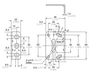
Material: Cold rolled carbon steel (SPCC)(Uni-chrome plated)
