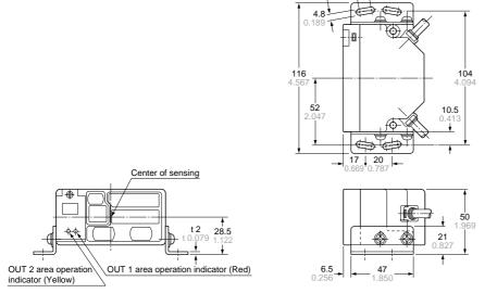
DIMENSIONS (Unit: mm in) The CAD data in the dimensions can be downloaded from the SUNX website: http://www.sunx.co.jp/
