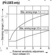
Correlation between external sensitivity adjustment input voltage and sensing range
