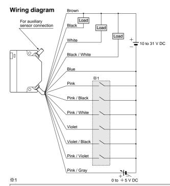
Non-voltage contact or NPN open-collector transistor
