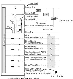
Symbols ... D: Reverse supply polarity protection diode Z<sub>D1</sub>, Z<sub>D2</sub>, Z<sub>D3</sub>: Surge absorption zener diode Tr<sub>1</sub>, Tr<sub>2</sub>, Tr<sub>3</sub>: NPN output transistor
