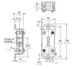
Material: Cold rolled carbon steel (SPCC)(Uni-chrome plated)
