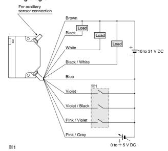
Non-voltage contact or NPN open-collector transistor
