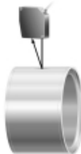
Detecting the seams of a metal drum
