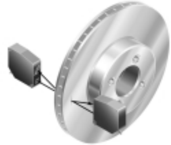
Detecting the presence of a resin coating
