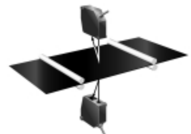
Measuring the thickness of rubber sheet
