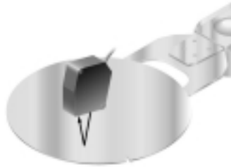
Measuring the eccentricity of a metal shaft
