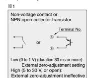
The external zero-adjustment input operation is independent of the state of the 'button operation effective / ineffective selection switch'.
