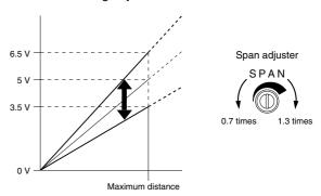
Note: Since the span adjustment can be done irrespective of the 'button operation effective / ineffective selection switch' position, do not operate the span adjuster after the adjustment.
