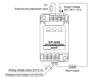
Note: After the wiring, make sure to fit the terminal covers. The terminal cover having a concave depression at the top should be fitted on the side having terminal Nos. 1 to 4.
