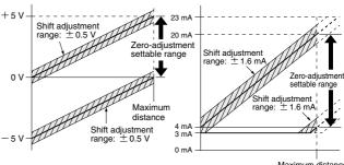
• Using the 'shift-up button' and the 'shift-down button', it is possible to adjust the offset value for the analog voltage output by  $\pm\,0.5$  V and that for the analog current output by  $\pm\,1.6$  mA.
