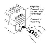
Note: Do not pull by holding the cable, as this can result in cable disconnection
