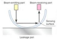
When there is no leakage The beam from the beamemitting part reflects off of the surface of the sensor and is transmitted to the beam-receiving part.
