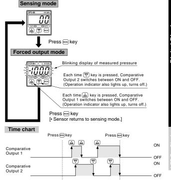
Sensing mode -Forced output mode – Sensina mode 🛶
